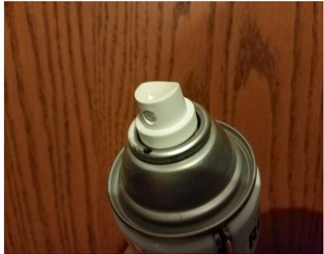
The dot on a spray can is used to show the position of the pickup tube in the bottom of the can. Position the nozzle toward the dot if spraying downward. If tilting the can upward, position the nozzle away from the dot.
